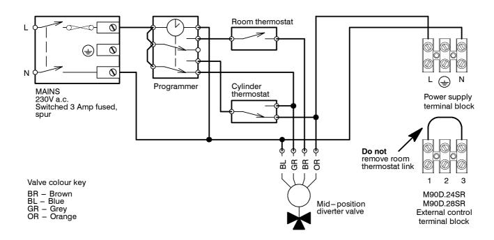
Fig. 6.18 - directly controlled boiler
