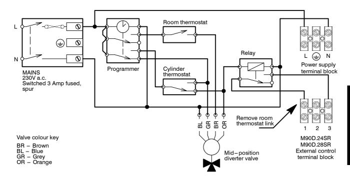
Fig. 6.17 - relay controlled boiler
